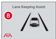
When the front-view camera does not detect the lane traveling in, the lanes are not illuminated gray
