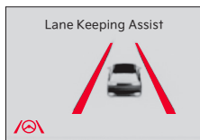
When the front-view camera detects the lane traveling in, both lanes are illuminated gray
