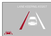
When the front-view camera detects the vehicle moving outside of the lane traveling in, a vehicle crossing lane indicator will blink, either on the left or right lane (as shown in both images above)
