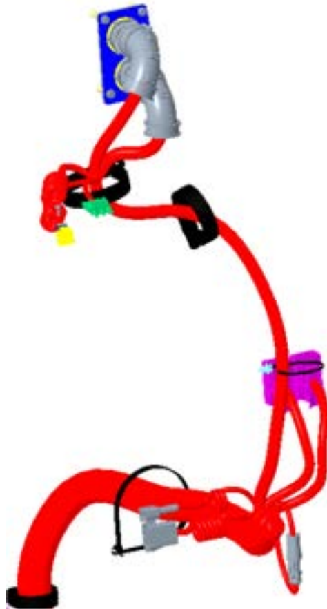
Detail View of Engine Compartment Body Connectors
