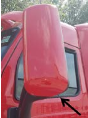
FIGURE 2-3: Aerodynamic Mirror OAT Sensor Location
