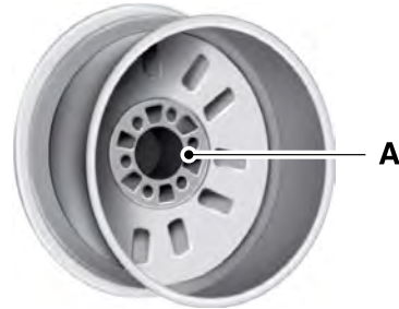
A Hub pilot bore.
