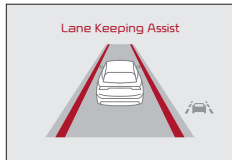
When the front view camera detects the lane the vehicle's traveling in, both lanes are illuminated
