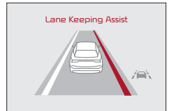
When the front camera detects the vehicle moving outside of the lane the vehicle's traveling in, a vehicle crossing lane indicator will blink, either on the left or right lane (as shown in both images above)
