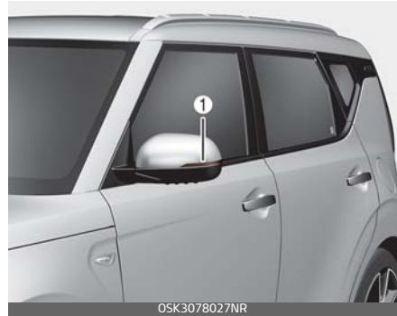
Light bulb position (Side)
