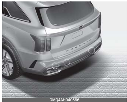
Rear ultrasonic sensors
