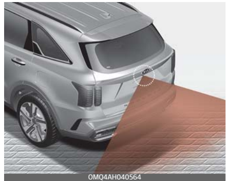
Rear ultrasonic sensors
