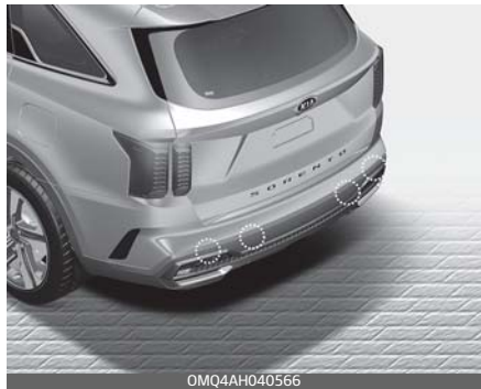
Rear ultrasonic sensors
