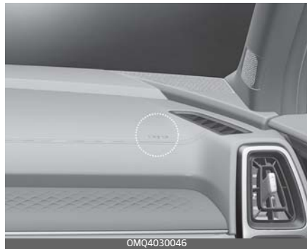
Passenger's front air bag
