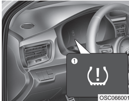
(1) Low tire pressure telltale/ TPMS malfunction indicator
