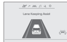
When the front-view camera does not detect the lane traveled in the lanes are not illuminated
