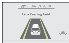
When the front-view camera detects the lane traveled in, both lanes are illuminated
