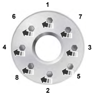
8-lug nut torque sequence
