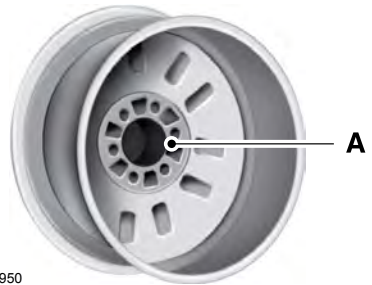
A Hub pilot bore.
