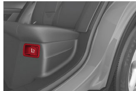
Seat Back Release Lever Below Rear Seat
