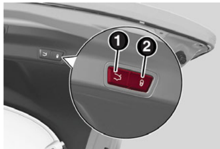
Power Liftgate/Lock Switches
