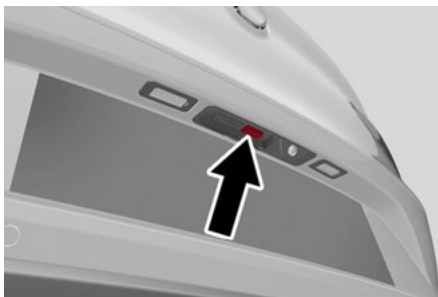
External Liftgate Release Switch
