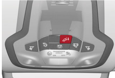
Volumetric/Anti-Lift Protection Button
