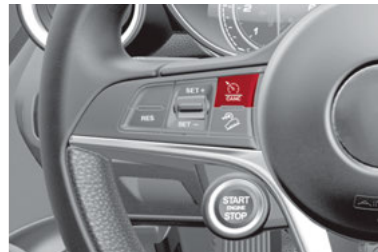
Cruise Control On/Off Switch
