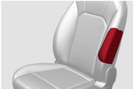
Front Supplemental Seat-Mounted Side Air Bag
