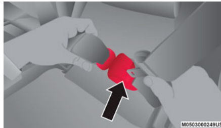
Detaching Mini-Buckle With Seat Belt Tongue
