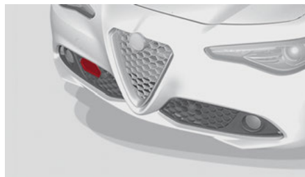
Front Fascia/Bumper Radar Location
