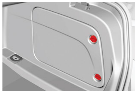
Battery Access Panel
