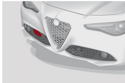
Front Bumper Radar Location
