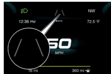
Lane Markings Not Detected
