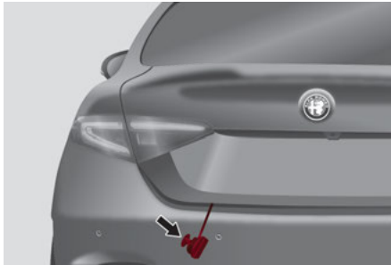
Manual Release Cord Shown With Trunk Closed
