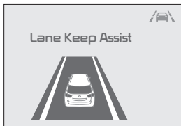
When the LKA sensor detects the lanes traveling in, the indicators are illuminated
