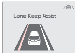
When the LKA sensor detects the vehicle moving outside of the lane the vehicle's traveling in, a yellow indicator will illuminate, either on the left or right lane
