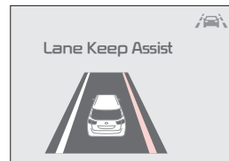
When the LKA sensor detects the vehicle moving outside of the lane the vehicle's traveling in, a yellow indicator will illuminate, either on the left or right lane
