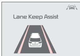
When the LKA sensor does not detect the lanes traveling in, the indicator will not illuminate
