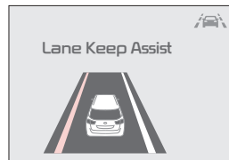
When the LKA sensor detects the vehicle moving outside of the lane the vehicle's traveling in, a yellow indicator will illuminate, either on the left or right lane
