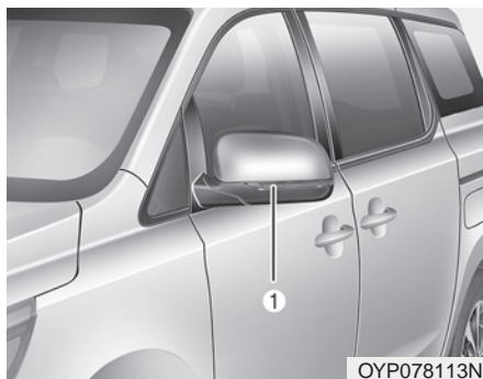
(1) Side repeater lamp (LED type)
