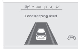
When the LKA sensor does not detect the lane traveled in, the lanes are not illuminated
