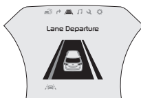
When the LDW sensor detects the lane traveling in, the lane is illuminated
