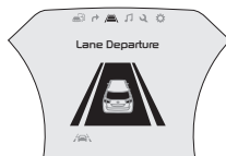
When the LDW sensor detects the lane traveling in, the lane is illuminated
