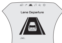
When the LDW sensor detects the lane traveling in, the lane is illuminated
