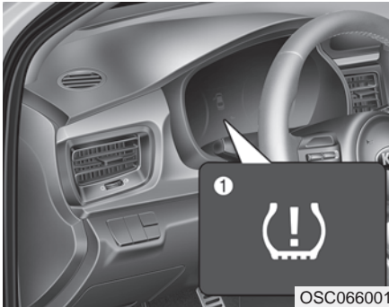
(1) Low tire pressure telltale / TPMS malfunction indicator
