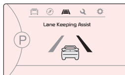
When the LKA sensor detects the vehicle veering outside of the lane traveling in, a yellow indicator will illuminate
