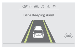
When the LKA sensor detects the lane traveled in, both lanes are illuminated
