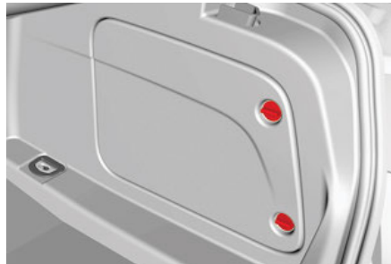
Battery Access Panel
