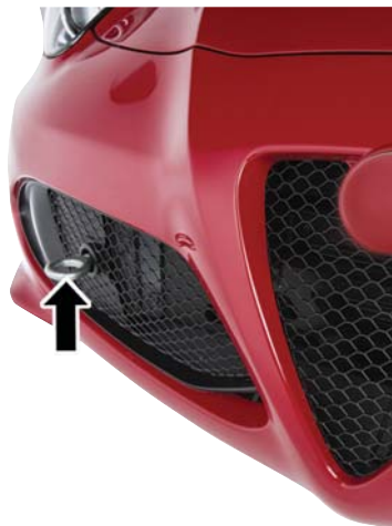
Front Tow Eye Installed
