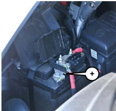
Positive Battery Post
