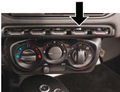
Door LED Lock Indicator
