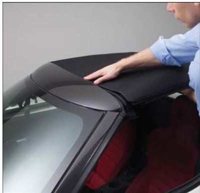
Installing Top Under The Vehicle Spoiler
