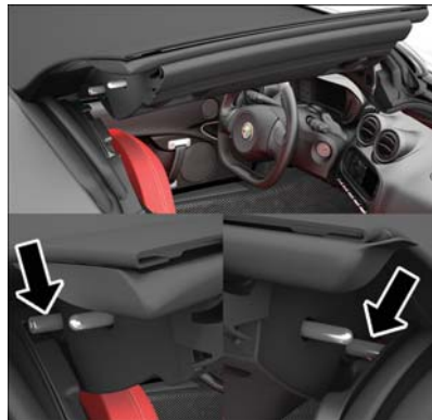
Locating Pins Seating In The Vehicle
