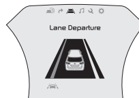
When the LDWS sensor detects the vehicle veering outside of the lane traveling in, a yellow indicator will illuminate the left or right lane that the vehicle's crossing (shown in both images above)
