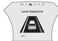
When the LDWS sensor detects the vehicle veering outside of the lane traveling in, a yellow indicator will illuminate the left or right lane that the vehicle's crossing (shown in both images above)
