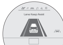
When the LKAS sensor detects the vehicle veering outside of the lane traveling in, a yellow indicator will illuminate either on the left or right lane (shown in both images above)
