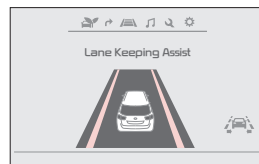
When the LKA sensor detects the lane traveling in, both lanes are illuminated
