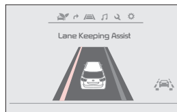
When the LKA sensor detects the vehicle veering outside of the lane traveling in, a yellow indicator will illuminate either on the left or right lane (shown in both images above)
