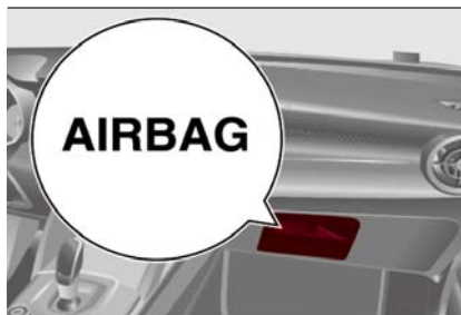
Passenger Knee Air Bag Location/Knee Bolster Location
