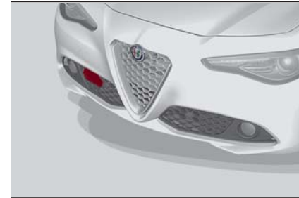
Front Bumper Radar Location
