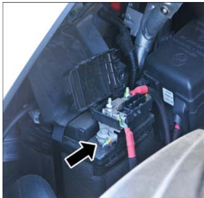
Positive (+) Battery Post
