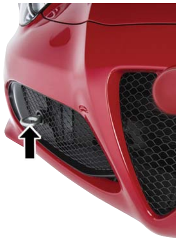
Front Tow Eye Installed
