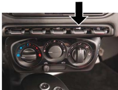
Door LED Lock Indicator
