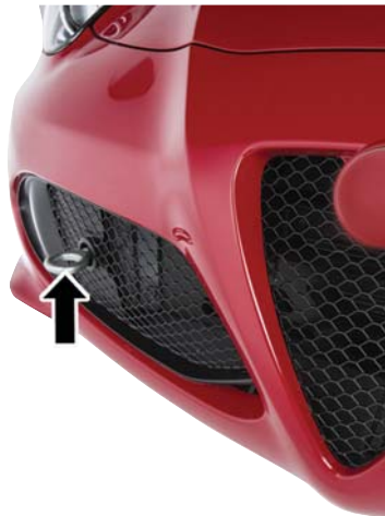
Front Tow Eye Installed
