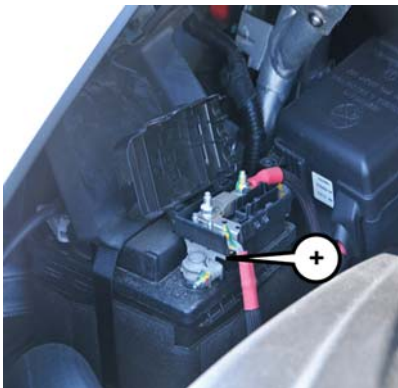
Positive Battery Post
