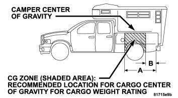
The tables on the following pages designate the Cargo Weight Rating and the Center of Gravity Zone for each vehicle listed.
