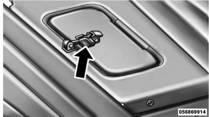
Manual Shut Off Valve Access Door
