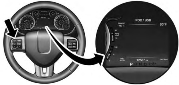
Instrument Cluster Display — Premium The Instrument Cluster Display features a driver-interactive display that is located in the instrument cluster.
