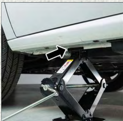
Front Jacking Location Engaged
