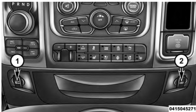
Power Outlets — Center Stack
