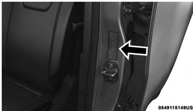
Example Tire Placard Location (B-Pillar)
