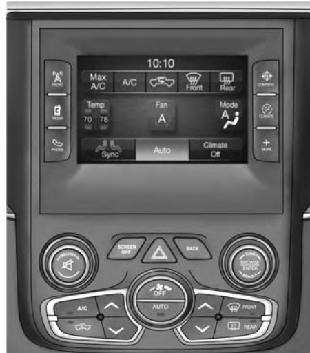
5.0 With Automatic Temperature Controls
