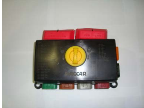
Figure 7.6.1 Pwer Distribution Center
