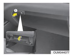
The glove box can be locked and unlocked with a master key. (if equipped) To open the glove box, push the button and the glove box will automatically open. Close the glove box after use.
