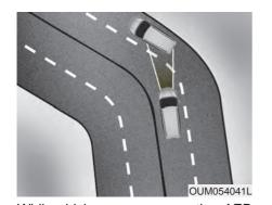
While driving on a curve, the AEB may recognize the vehicle in front in the next lane. Exercise caution, and, if necessary, depress the brake pedal. Or, depress the accelerator pedal to maintain the driving speed. Always, take a look around the vehicle for your safety.
