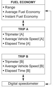
To change the trip mode, scroll the TRIP scroll switch  $(\triangle/\nabla)$  in the trip computer mode.
