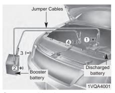
Connect cables in numerical order and disconnect in reverse order.
