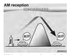
AM broadcasts can be received at greater distances than FM broadcasts. This is because AM radio waves are transmitted at low frequencies. These long distance,low frequency radio waves can follow the curvature of the earth rather than travelling straight. In addition, they curve around obstructions resulting in better signal coverage.
