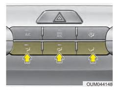
The mode selection button controls the direction of the air flow through the ventilation system.
