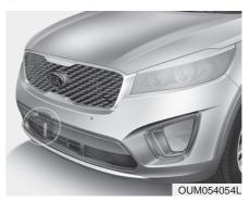
The sensor cannot maintain proper distance from the vehicle in front when the sensor lens is obscured by foreign substances, such as snow and rain, which will adversely affect performance. It may even temporarily cancel the AEB. Always keep the sensor clean.
