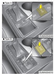
Engine power can be delivered to all front and rear wheels for maximum traction. AWD is useful when extra traction is required, such as, when driving on slippery, muddy, wet, or snow-covered roads.
