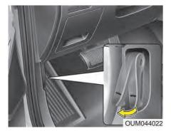
1. Pull the release lever to unlatch the hood. The hood should pop open slightly. Open the hood after turning off the engine on a flat surface, shifting the shift lever to the P (Park) position and setting the parking brake.
