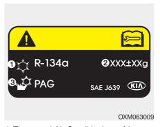
\* The actual Air Conditioning refrigerant label in the vehicle may differ from the illustration. Each symbol and specification on the air conditioning refrigerant label is represented below;
