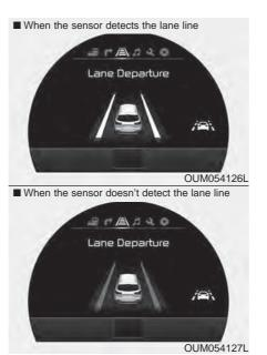
If the system detects that your vehicle is leaving the lane when the LDWS is operating and vehicle speed exceeds 40 mph (64 km/h), the warning operates as follows:
