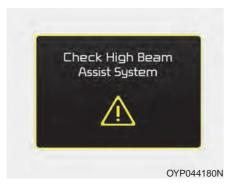
This warning message illuminates if there is a malfunction (burned-out bulb or circuit malfunction) with the headlamp. In this case, have your vehicle inspected by an authorized Kia dealer
