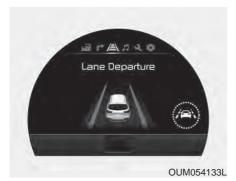
To operate the LDWS, press the button with the engine start/stop button in the ON position. The indicator illuminates on the cluster. To cancel the LDWS, press the button again.
