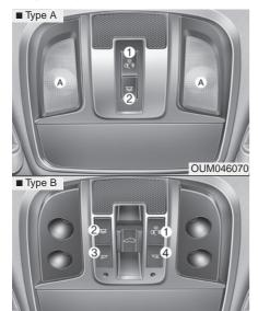
• Press the lens (A) to turn the map lamp on.
