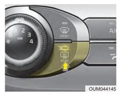
The defroster heats the window to remove frost, fog and thin ice from the rear window, while the engine is running.
