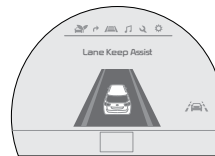
When the LKAS sensor does not detect the lane traveling in the lanes are not illuminated
