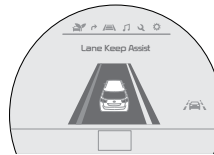
When the LKAS sensor detects the vehicle veering outside of the lane traveling in, a yellow indicator will illuminate either on the left or right lane (shown in both images above)
