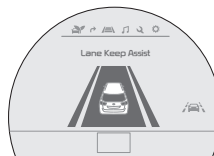
When the LKAS sensor detects the lane traveling in, both lanes are illuminated
