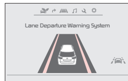
When the LKAS sensor detects the lane traveling in, both lanes are illuminated
