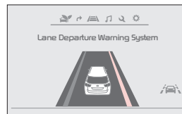
When the LDWS sensor detects the vehicle veering outside of the lane traveling in, a yellow indicator will illuminate either on the left or right lane (shown in both images above)
