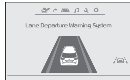
When the LKAS sensor does not detect the lane traveling in the lanes are not illuminated
