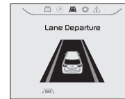
When the LDWS sensor does not detect the lane traveling in the lanes are not illuminated
