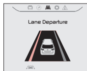
When the LDWS sensor detects the vehicle veering outside of the lane traveling in, a yellow indicator will illuminate either on the left or right lane (shown in both images above)
