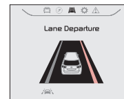
When the LDWS sensor detects the vehicle veering outside of the lane traveling in, a yellow indicator will illuminate either on the left or right lane (shown in both images above)
