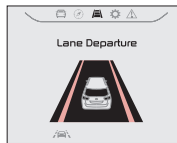
When the LDWS sensor detects the lane traveling in, both lanes are illuminated
