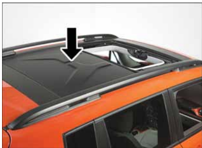
Installing Rear Panel
