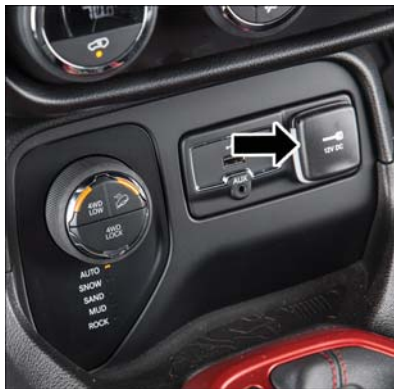
Front Power Outlet
