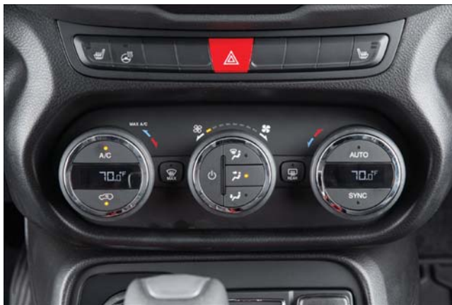
Automatic Temperature Controls (ATC)
