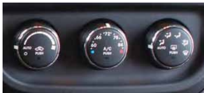
Automatic Temperature Controls
