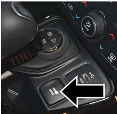
Front Power Outlet
