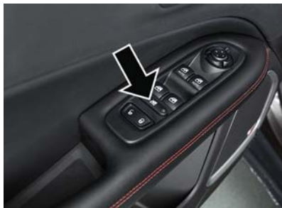
Window Lockout Switch
