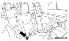
Inserting Latch Plate Into Buckle
