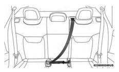
Inserting Latch Plate Into Buckle
