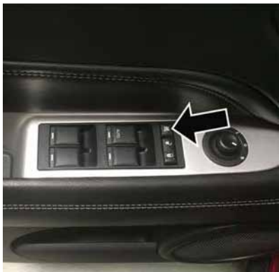
Window Lockout Switch
