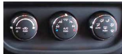
Automatic Temperature Controls
