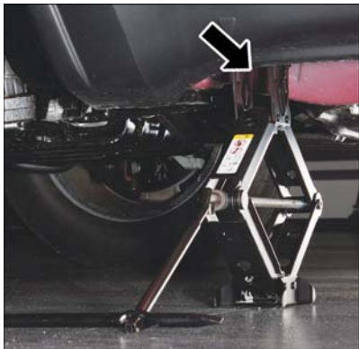
Front Jacking Location
