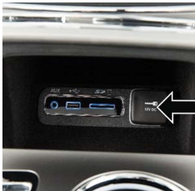
Front Power Outlet
