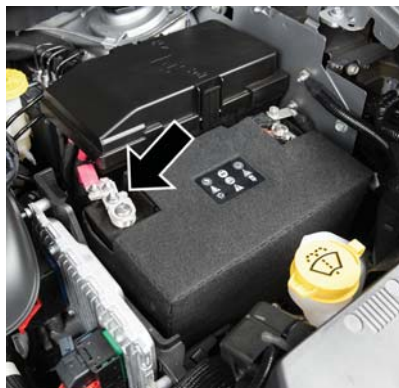
Positive Battery Post
