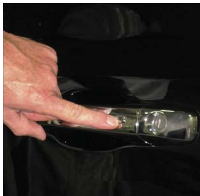
Push The Door Handle Button To Lock
