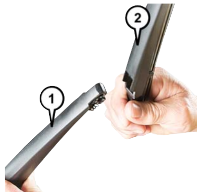
Wiper Blade Removed From Wiper Arm
