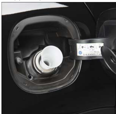
Fueling With Emergency Fuel Fill Funnel
