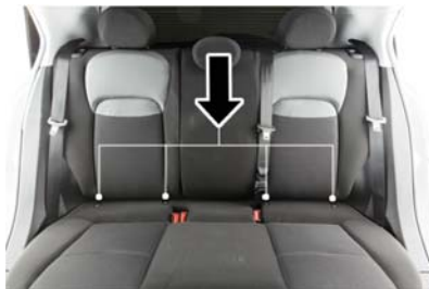
Lower Anchorage Location
