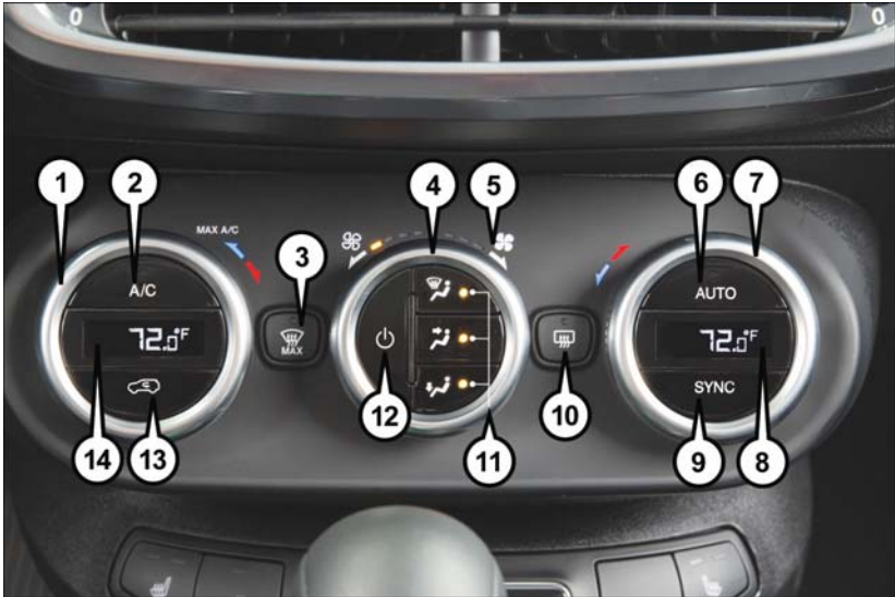
Automatic Temperature Controls (ATC)
