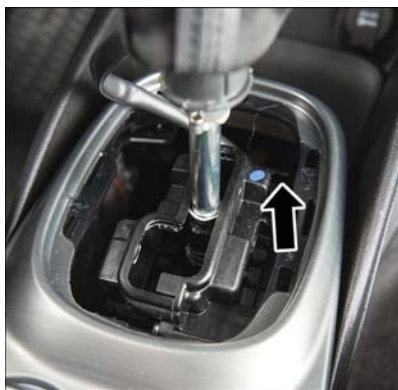
Gear Selector Override Location
