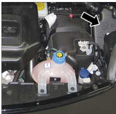
Front Distribution Unit
