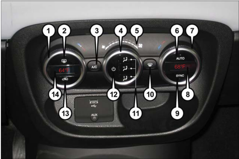
Automatic Temperature Controls (ATC)
